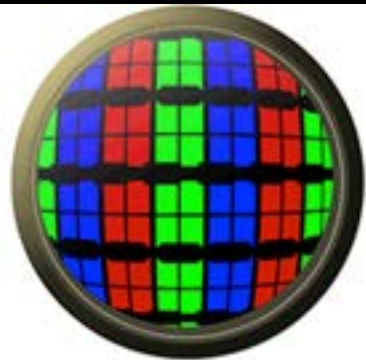
3 COLOR Red, Green and Blue sub-pixel representation
